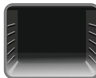
**Lower Heating Function:** The oven's thermostat and warning lights will switch on and the lower heating element will start operating. The lower heating function
