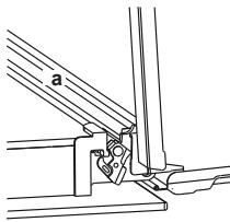
3. Close the door until it is almost in the fully closed position, and remove the door by pulling it towards you.
