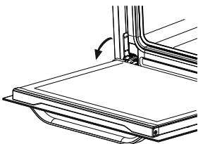
2. Open the locking catch (a) (with the aid of a screwdriver) up to the end position.
